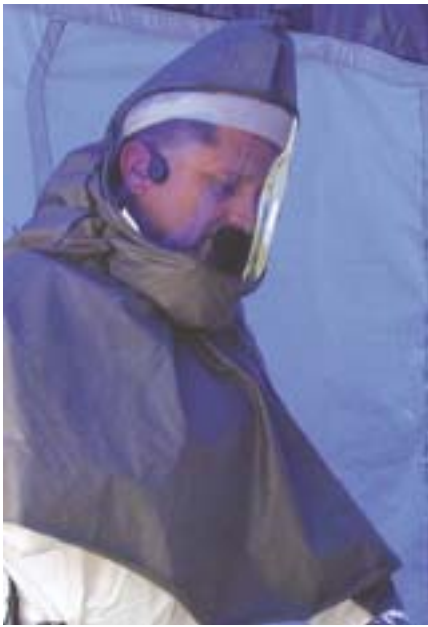
“Temple-transducer” style two-way radio headset stays in place under PAPER hoods.
