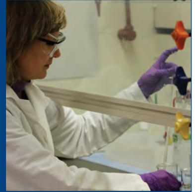
The fume hood is often the primary control device for protecting laboratory workers when working with flammable and/or toxic chemicals.
