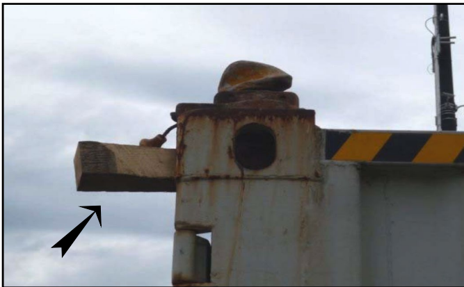
Wedge inserted into a container (side view).
