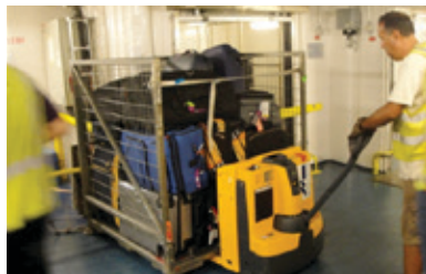
Photo above shows use of compact electric pallet jack aboard a ship.
