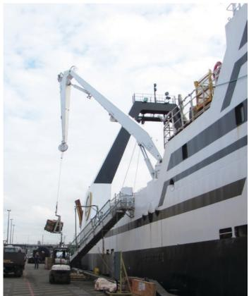
Shipboard pedestal cranes are used to move a wide range of materials safely and efficiently.
