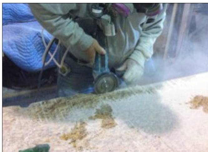
Cutting stone, as pictured, generates dangerous crystalline silica dust that can become trapped in lung tissue and cause silicosis.
