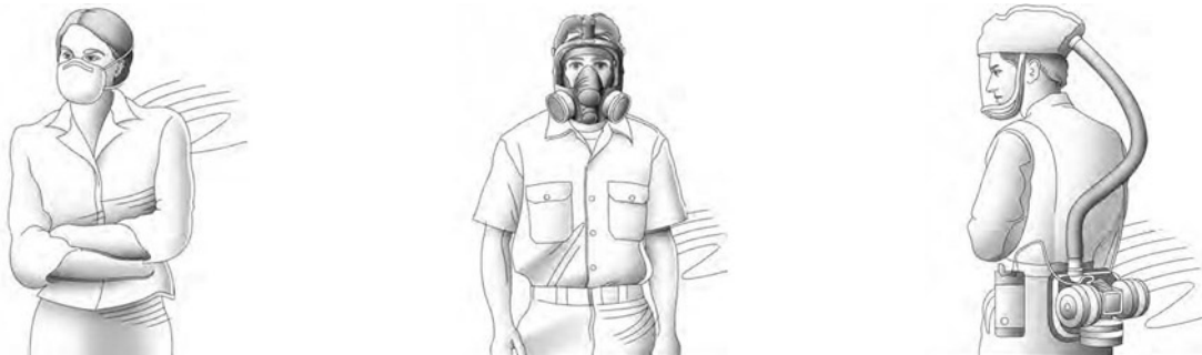
The workers shown above are wearing a NIOSH-approved N95 filtering facepiece respirator (left), a full facepiece elastomeric respirator (center), and a loose-fitting powered air-purifying respirator (PAPR) (right).
