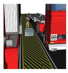
Traffic Lanes – are provided to guide and align container haulage equipment operating under cranes. Traffic lanes should be wide enough so that haulage equipment never enters the safety zone. Drivers should ensure that equipment stays within the traffic lane. Drivers should also control their speed while passing workers in safety zones.
