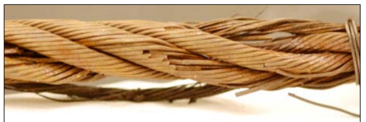
Failed 7/8" load line close-up. Note the broken wire strands.
