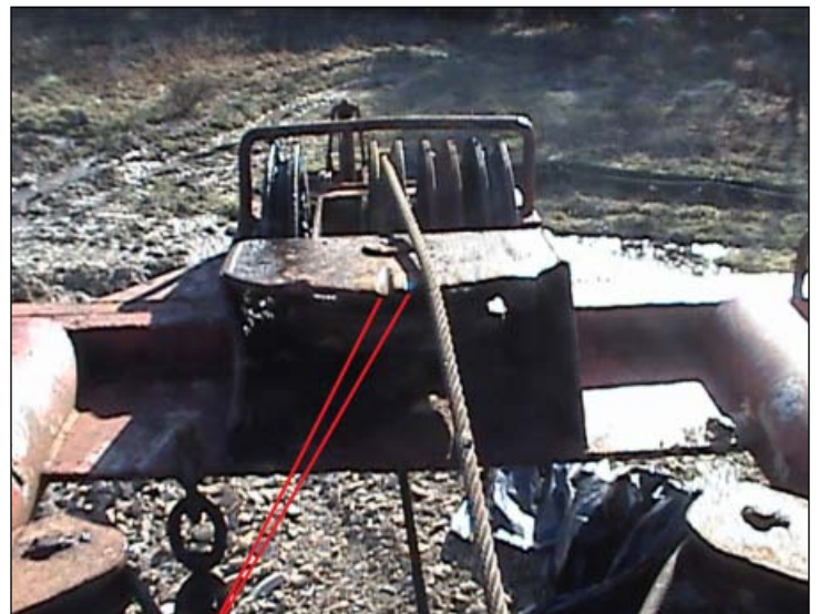
Wear marks in draw-works guard from failed line.
