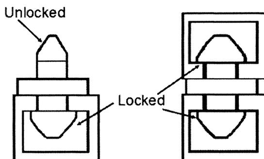
Figure 2—Interbox Connections (Source: Ex. 11-6H)
