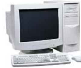
Hidden sources of contamination: Desktop computers and other objects with internal fans that draw air into the case may have filters or electrostatic devices to control dust intake.
