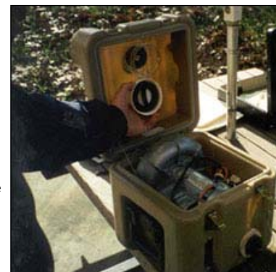
HEPA filters can be attached to high-volume vacuums such as this.
