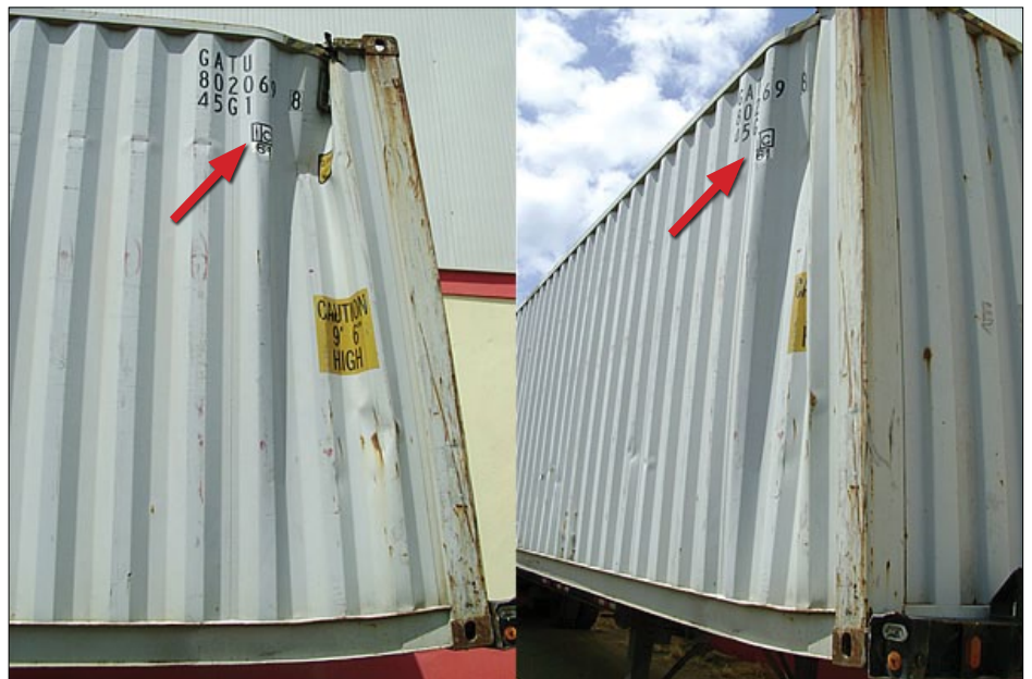
Figure 1: Intermodal container with structural damage.
